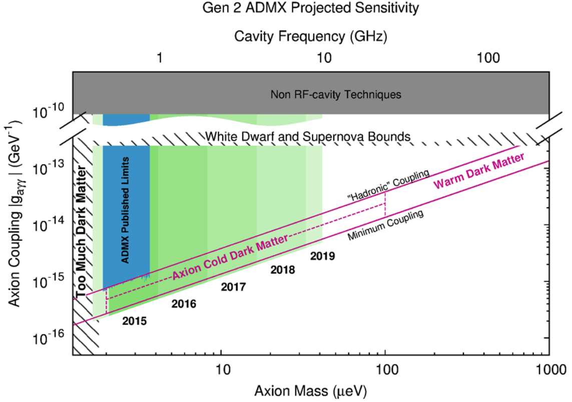
Figure 25: A graph of g_{A\gamma\gamma} ( \text{GeV}^{-1} ) vs. m_A ( \mu\text{eV} ) the projected sensitivity of the next stage of ADMX [93]. The sensitivity the ADMX-HF apparatus is also displayed.
