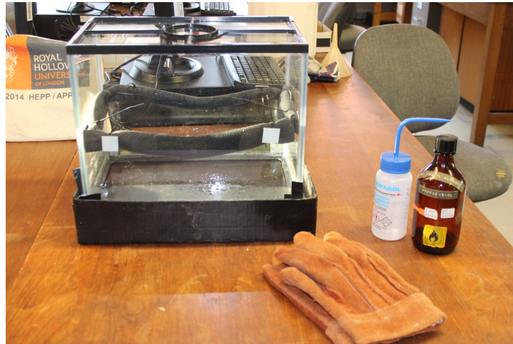
Figure 1: Photo of the final setup of the 'homemade' cloud chamber.
